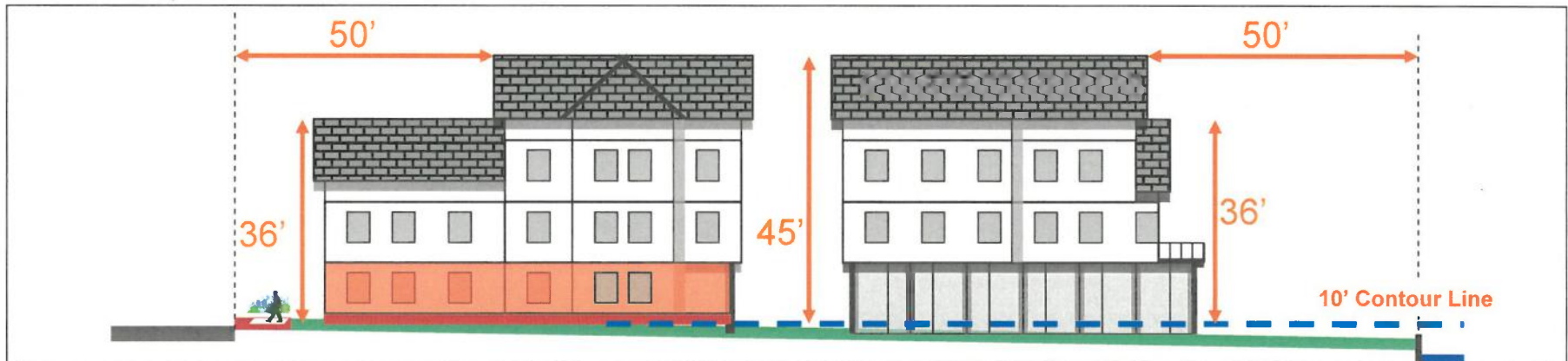
ILLUSTRATION 6-12.3A – Building Height Regulations (Showing height bonus allowed if first floor of building facing the street is restricted to Eating Establishments and/or Retail Commercial Uses)
